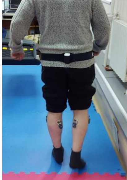
Fig. 2. Positioning of the G-Walk sensor in the area of S1 (os sacrum) and the FREE EMG electrodes on the m.tibialis anterior and m.gastrocnemius medialis of the examined person.
