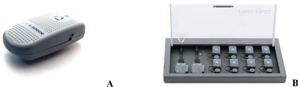
Fig. 1. The equipment used to assess the electromyographic and kinematic characteristics of gait A) G-Walk sensor and B) Bluetooth electrodes of FREE EMG of BTS Co. Italy
